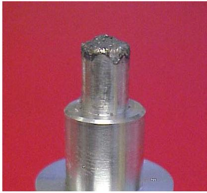
Fig. 3. Eroded aluminum cathode after electrothermal gun operation with energy deposition of 96 kJ.
